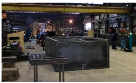
Linkflote pontoon being manufactured in the VolkerBrooks workshop
